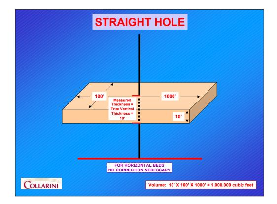
In this slide, our volume remains horizontal. Our well is vertical; therefore, the measured thickness equals the TVT and no correction must be made. Anytime the bed dip is zero, no true vertical thickness correction needs to be made.
