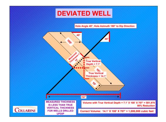
Now, let's drill a directional well with a hole angle of 45 degrees drilled perpendicular to our volumes dip direction.
