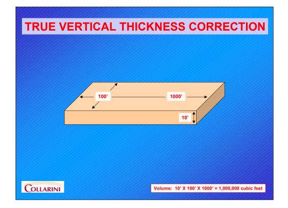
Two of the questions asked most frequently are: "What is the difference between measured thickness and true vertical thickness?" and "How does the difference affect reservoir volume calculations?" The following presentation is an example of how not making a proper correction can affect volumetrics.
