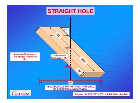
Pretend we're drilling on the flank of a salt dome. Let's rotate our volume until it is at a 45 degree angle. We'll leave the well vertical.
